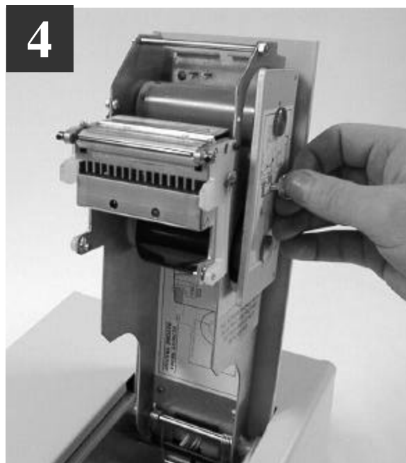
4 Open the Dye Film package. Fit the dye film on the lower boss, observing the correct orientation of the dye film. Fit the empty take-up core on the upper boss, observing the correct orientation of the notches on the Take-up Core.
